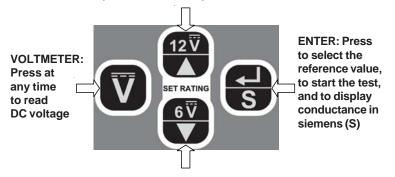
DOWN ARROW: Press for 6-volt batteries and to scroll to the reference value (20 to 1200 siemens).
